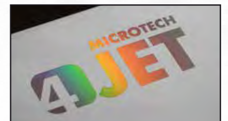
Fig. 7: Photograph of a processed workpiece: The micro-texturing results in a macroscopic shimmering effect of the processed areas.
