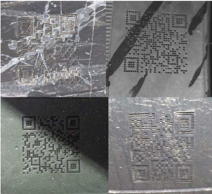
Figure 3: Typical QR captures from field testing. The codes are non-legible with ZXing however, could be de-coded after image pre-processing.
